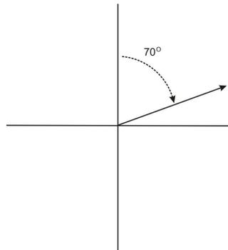
It is important to keep in mind that angles in navigation problems are measured this way, and not the same way angles are measured in the unit circle. Further, angles in navigation and surveying may also be given in terms of
