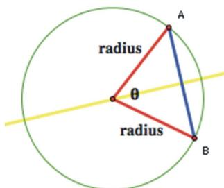
We can now use a simple sine ratio to find half the chord, called  $c$  here, and double the result to find the length of the chord.
