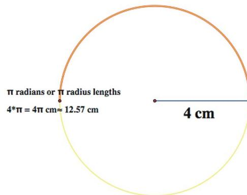
This results in a formula that can be used to calculate the length of any arc.
