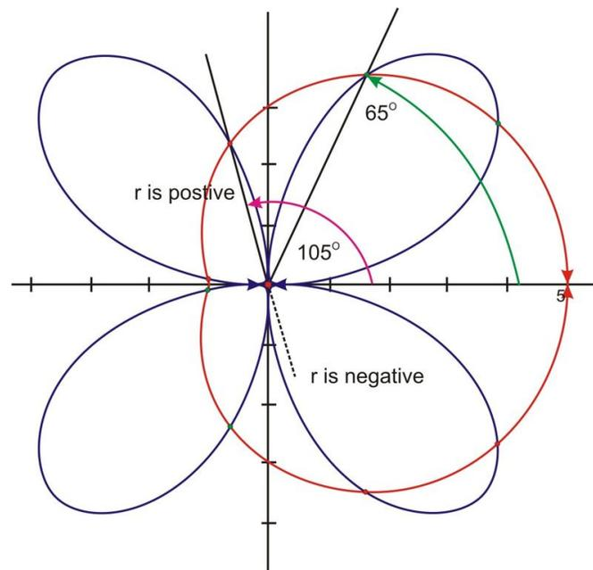
There appear to be 8 intersection points between the limaçon, and the rose. However, the true points of intersection are the two points in the first quadrant and the two points in the third quadrant. At the other four intersection points, the  $r$ - values on the rose are negative.
