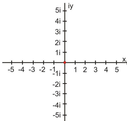
This is a model of the **complex plane**. The horizontal number line is called the **real axis**. Every real number is the coordinate of a point on this axis. The vertical line is called the **imaginary axis**. Each pure imaginary number or  $i$ - number is the coordinate of a point on the axis.
