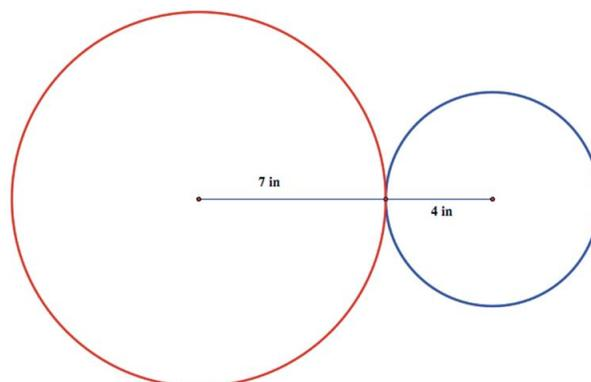
Because the blue gear performs one complete rotation, the length of the arc traveled is:
